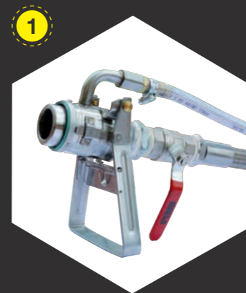
Complete connection system disposal, 3-PIN Used product coupling with shut-off valve and 3 m solvent-resistant \frac{3}{4} " hose and vapour return line Art. no.: 299010
